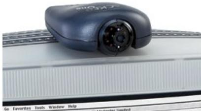
Mounting on a desktop computer places Tracker One flat on the top of your computer monitor with the sensor pointing straight towards you.
