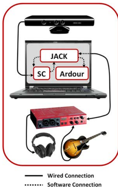
Figure 3. Configuration of the system's hardware and software components.
