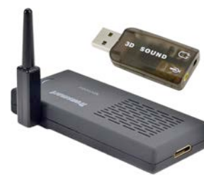
Figure 3. Citygram’s Android mini-PC, audio interface solution.
