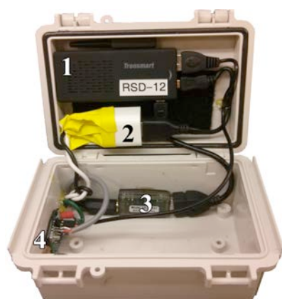
Figure 6. Complete fixed-RSD (1 – mini PC, 2 – power supply, 3 – USB audio interface, 4 – MEMS mic with board)
