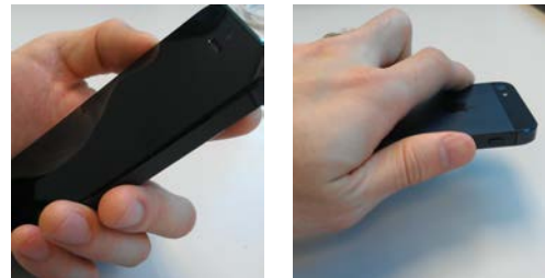
Figure 4. Gravity Y gesture (on the left), which is used for controlling note velocity, leading to a smaller velocity with a larger angle to the horizontal plane; Gravity Z gesture (on the right), which is used for quitting the current keyboard to reset everything again
