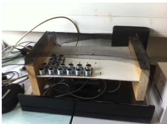
Figure 3. Ultrasound matrix, for eight keys.
