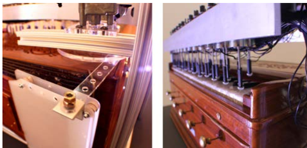
Figure 2. Kritaanjli's keyboard playing mechanism (right) and bellows pumping system (left). Both are affixed to Kritaanjli's t-slot aluminium chassis.
