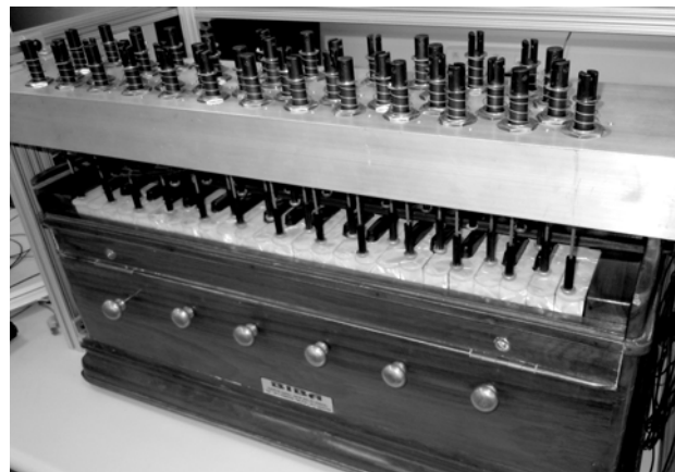
Figure 3. Kritaanjli's keyboard player: each of the 44 solenoid actuators is positioned above a key. Upon actuation, the solenoid's plunger extension depresses its key. The width of the solenoids necessitated their staggered placement above the keyboard.
