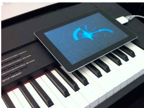
Figure 4. TC-Data running on an iPad, connected to an external MIDI interface. The MIDI controller data can be merged with the keyboard output.
