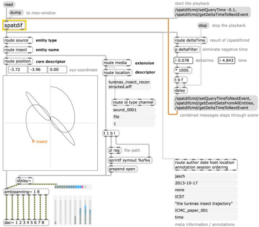
Figure 3: Implementation of SpatDIF in a MaxMSP external (marked in yellow), demonstrating the playback of the Lissajous trajectory from John Chowning’s ‘Turenas’.
