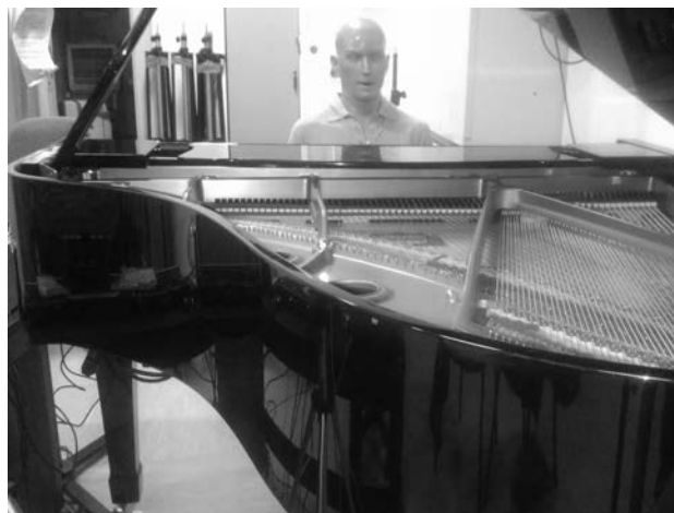
Figure 1: Setup for loudness estimation on the grand piano (PD) using a KEMAR mannequin.
