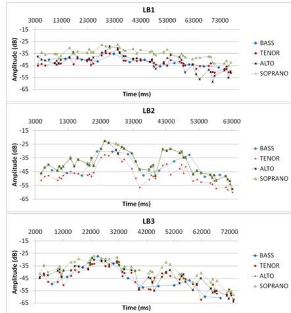
**Figure 5.** Amplitude curves for each voice in examples (a) LB1, (b) LB2 and (c) LB3.
