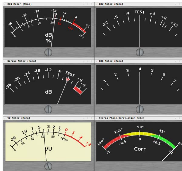
Figure 2. Various meter-types from the meter.lv2 plugin bundle fed with a -18 dBFS 1 kHz sine wave. Note, bottom right depicts the stereo phase correlation meter of a mono signal.
