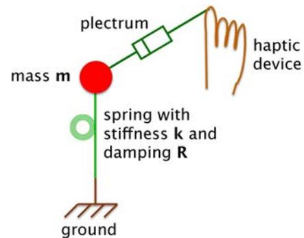
**Figure 1.** A resonator is formed by a mass  $m$  connected to ground via a spring ( $k, R$ ). A human can pluck this resonator by way of a virtual plectrum and haptic device.
