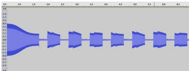
**Figure 8.** String that was plucked at  $t=0$  sec when tuned to a note with a typical “audible” fundamental frequency, which was then dropped to about 0.4Hz starting at time  $t=1.7$  sec.
