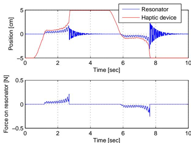
**Figure 10.** Above: position of a frequency-modulated resonator (in blue) and a haptic device (in red), below: force between the frequency-modulated resonator and the haptic device as exerted by the plectrum.
