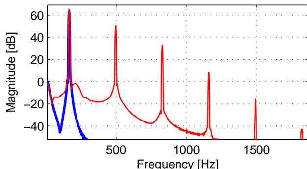
**Figure 4.** Magnitude response of a simple plucked resonator (e.g.  $d = 0$  in thick blue) overlaid over a frequency-modulated plucked resonator (e.g.  $d = 0.95$  and  $f_m = 4.03f_c$  in thin red). Note that the energy near 0Hz comes as a result of the model’s excitation via a virtual plectrum.
