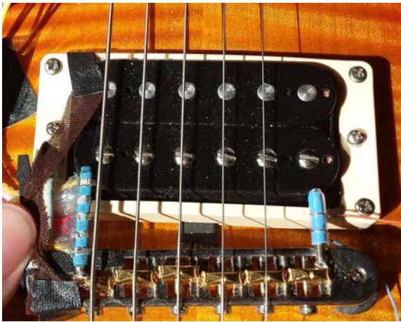
Figure 6. Pressure sensor soldered on the saddle of a Les Paul bridge, sensing palm pressure along the string.
