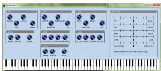
Figure 5. The interface of the test system. The graphical user interface mimics the physical appearance of a simple analog synthesizer, thus creating compatibility with standard commercial systems. The evaluation unit is used to collect user data during the naming process.
