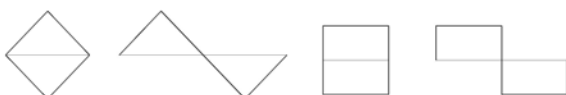
Figure 3. A triangle and a square wave or tetragon waves with start phase 0 and \pi/n derived from a square
