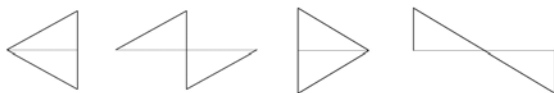
Figure 2. Sawtooth waves or trigon waves with start phase 0 and \pi/n derived from a triangle.
