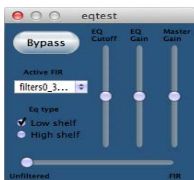
Figure 5. Screenshot of the equalizer VST plugin. The plugin displays a cross-fader between unfiltered and filtered signal, a menu for filter choosing coefficients, and an additional low/high shelf EQ with cutoff and gain functions.
