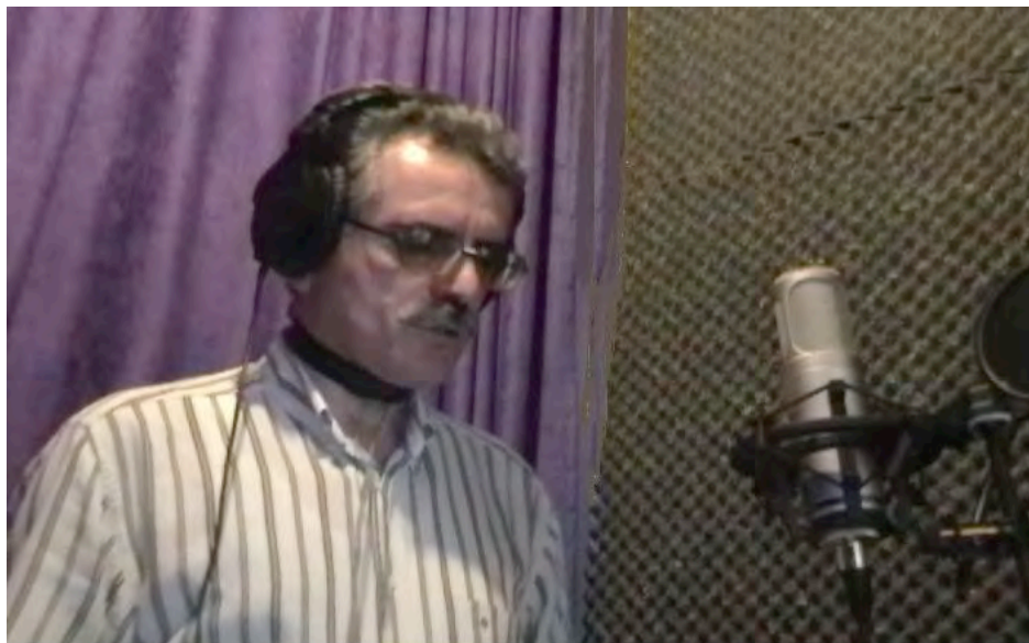
Figure 4. Experimental setup showing a participant with the microphone, the electroglottographic sensors and the headphones during the recordings.
