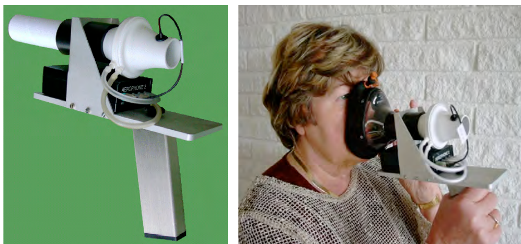
(a) (b) Figure 2. The Aerophone II apparatus (a) and its usage for the aerodynamic measurements of the voice (b).
